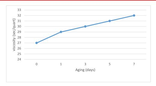
**Figure 9**: Viscosity as a function of aging
